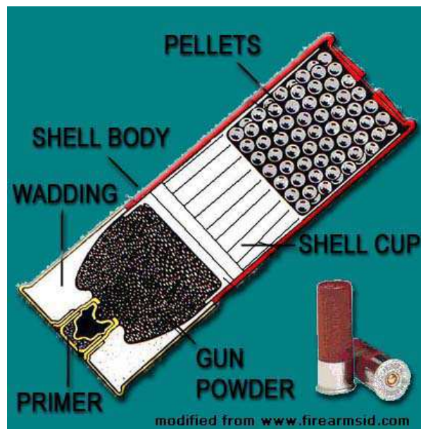
Figure 1. Longitudinal section of a modern shotgun shell
